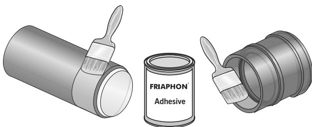
Apply adhesive all over faces with brush
